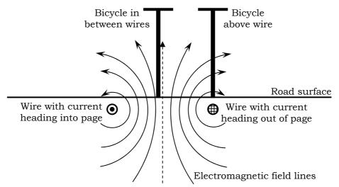
For a large wide object like a car, it is not particularly difficult to get some part of the vehicle slicing the EMF and triggering the detector (the larger mass of metal also causes a greater change in inductance).
