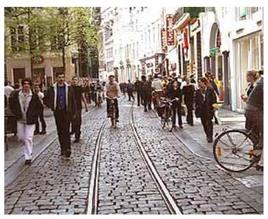
of pedestrians and cyclists are **in excess of 180/hour per metre width** of paved area, a segregated cycle path should be provided.
