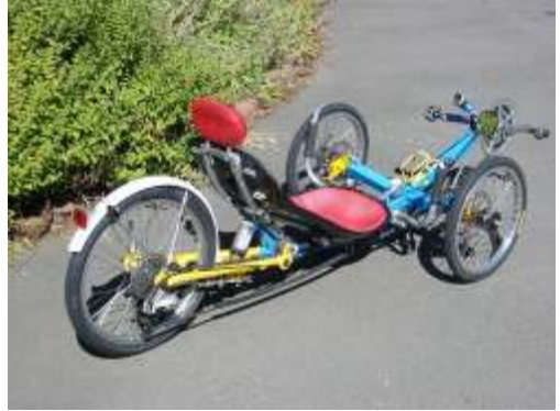
A recumbent tadpole tricycle, based on an overseas design. Built by Bruce McDowell of Christchurch.
