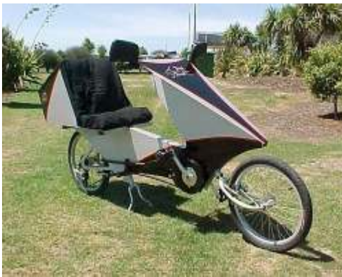
A semi-faired long wheel base recumbent, currently undergoing development in NZ by Feet First HPVs
