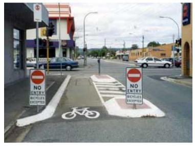
Another way to achieve a similar effect, particularly in local area traffic management schemes, is to create a "false" one-way entrance. This allows either entry only or exit only to a two-way street for motorists at one end, but lets cyclists bypass this restriction. The picture above shows an example from Australia, where only cyclists are allowed to exit the street here (with a cycle signal provided at the intersection).
