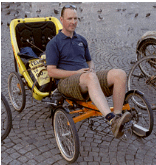
A 4 wheel recumbent with child (or luggage!) seat.
