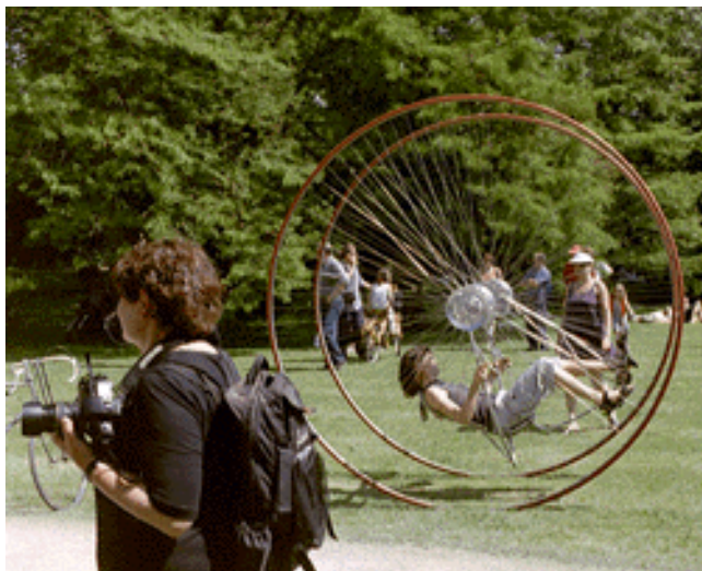
The twin-penny farthing recumbent? The bike is steered by independently braking the wheels.
