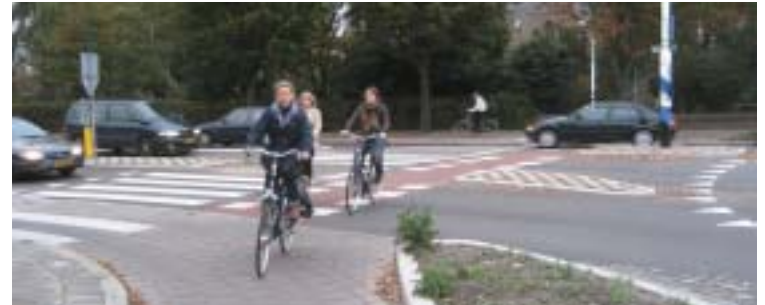
Cyclists and pedestrians at roundabouts in Holland have right-of-way on dedicated paths on the outer edge
